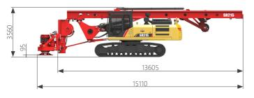
Efficient and flexible: Widely used in small dia. & deep borehole construction in civil engineering, high main hoist lifting up and down speed, high verticality of finished borehole, high working efficiency in civil construction.
