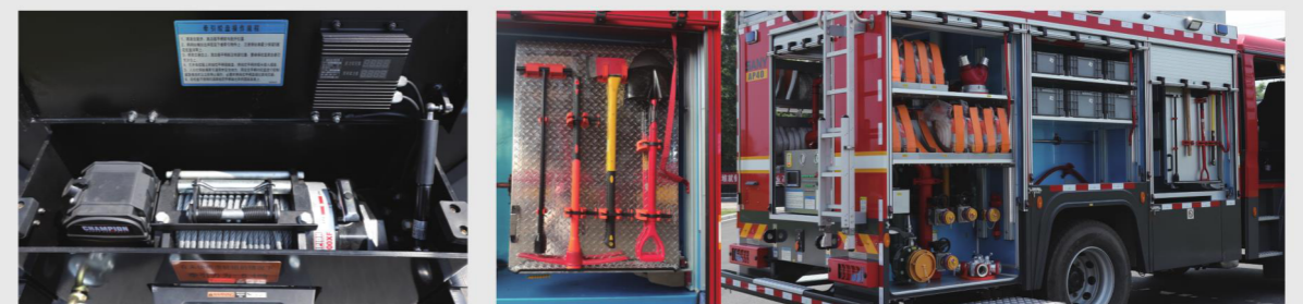
◆ American champion electric winch, maximum pull 5.4 tons
