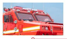
Anti-smash: Anti-smash: The frame-type independent cab can resist the vertical load impact of 100kg steel ball which falls from 20m height.
