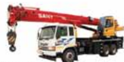
SPC250 Maximum Load Capacity: 25t Telescopic Boom: 4 Sections, 10.22-31.5m
